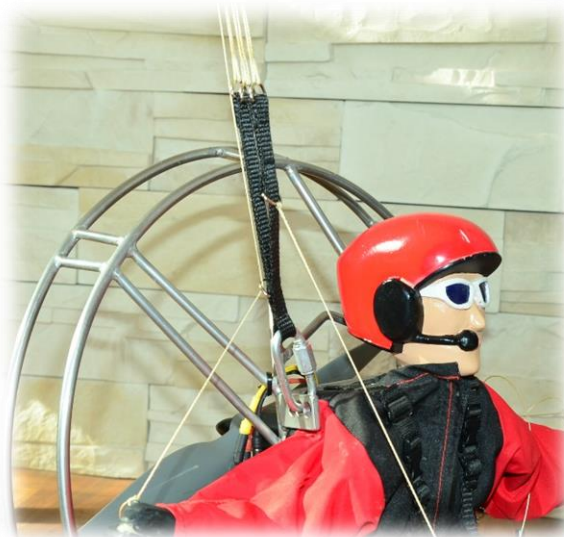
tie the line into D-ring
